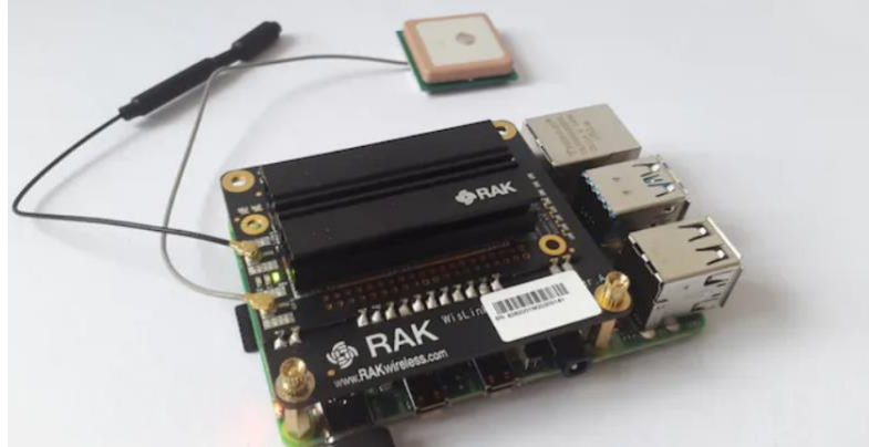
Figure 47: Shows the implementation of the Gateway design
